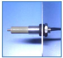
Step 2.1.3 Screw the intermediate pipe of the cable gland (incl. lamellar insert and sealing ring) at the Heat Detector and tighten afterwards the dome nut (see Figures)
